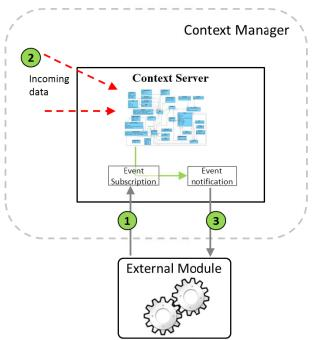
Figure 2 – Integration between the Context Manager and a generic external module relying on the subscription-notification mechanism.
