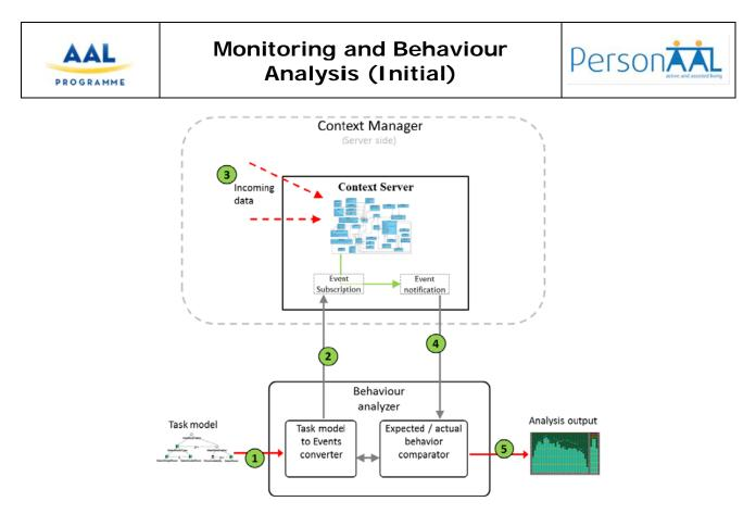
Figure 5 – Architecture of the integration between the Context Manager and the behaviour analysis system.
